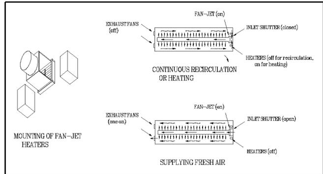
**Figure 5.** Schematic views of Fan-Jet Poly-Tube Systems.
