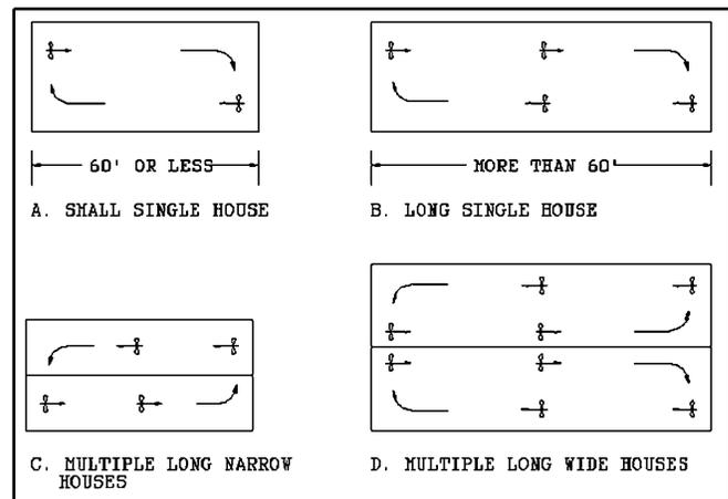
**Figure 1.** Typical arrangements for fans for horizontal convection air circulation systems.
