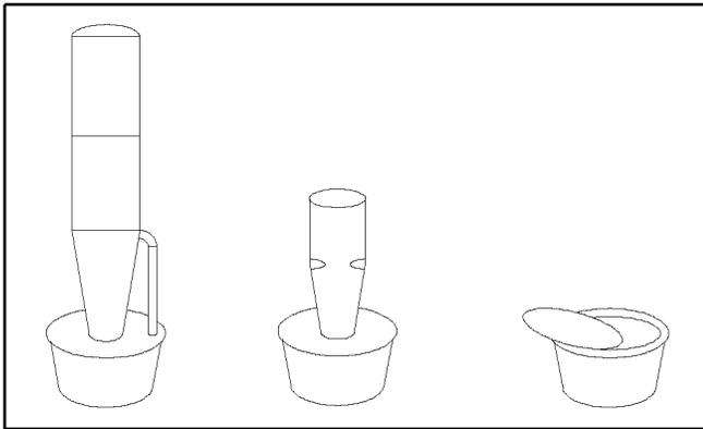
**Figure 3.** Radiant heaters of these types are not recommended for greenhouse heating.
