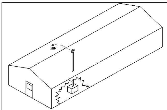
**Figure 2.** All greenhouse heating units should be vented to the outside. Top of vent sack should be at least 48" above the roof peak.
