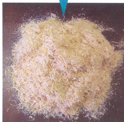
Figure 1. Pine tree chips can be further ground with a hammer mill to produce a substrate that show promise as an alternative to peat moss and pine bark. (Photos: Robert Wright)
